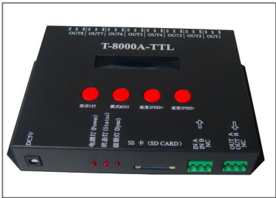
SD Card programe controller. SMD Capacity supports 128MB-32GB
