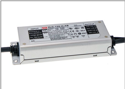
Order code: XLG-150-24-A AC100-305V DC24V 150W IP67, Global certification. Non Dimmable.
